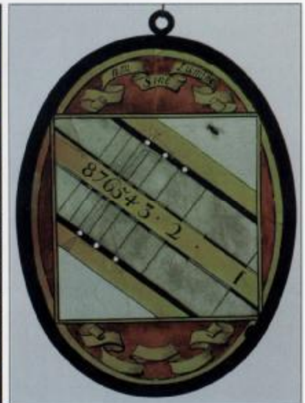
Fig. 6. The Non Sine Lumine dial, a direct west dial designed like a mathematical scale; the style of the inscription appears on a number of dials attributed to John Oliver. (Private collection).
